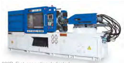
FB-200R, First-generation dedicated pen-making two-component IMM in 2003
