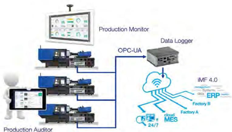
Figure 2. iMF 4.0 system structure
