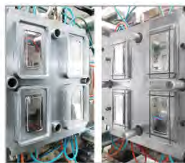
Figure 4. Cover mold with four cavities
