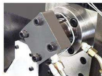
轉盤定位安全插銷 Rotary Platen's Position
